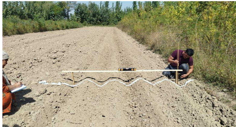
Figure 4. Determination of Ridge Height and Its Transverse Profile
